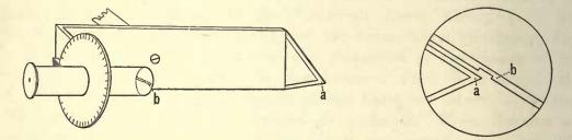
On the eyepiece, about 3 in. from the eye towards the V is a thin bar, b, with a notch at its middle point, which can turn about the line in which the instrument is pointing.
